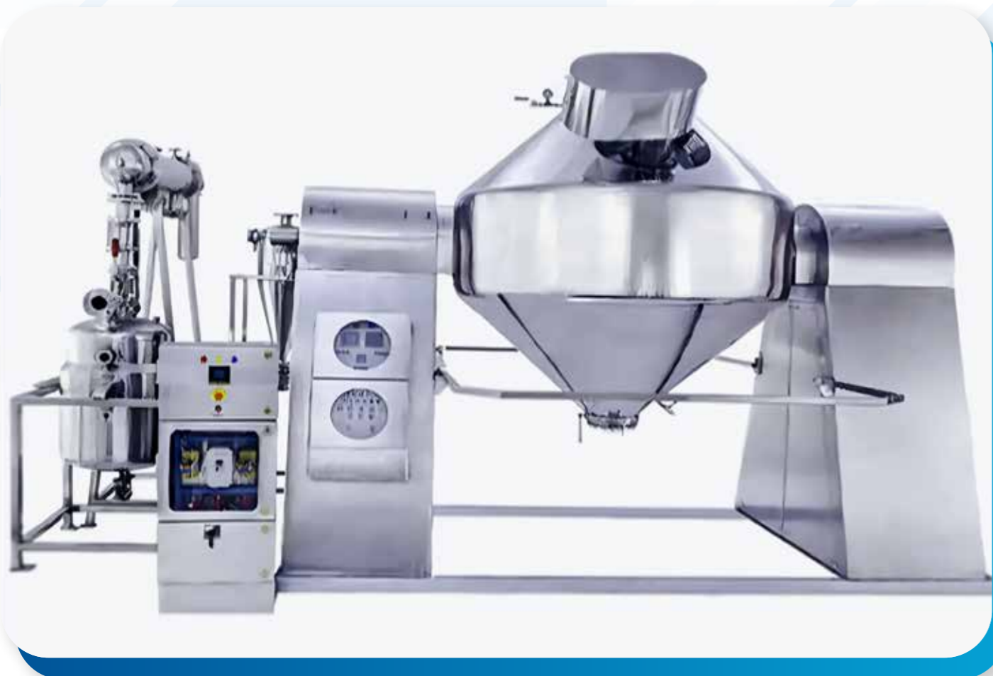
Fig. 4: Typical Vacuum Dryer
