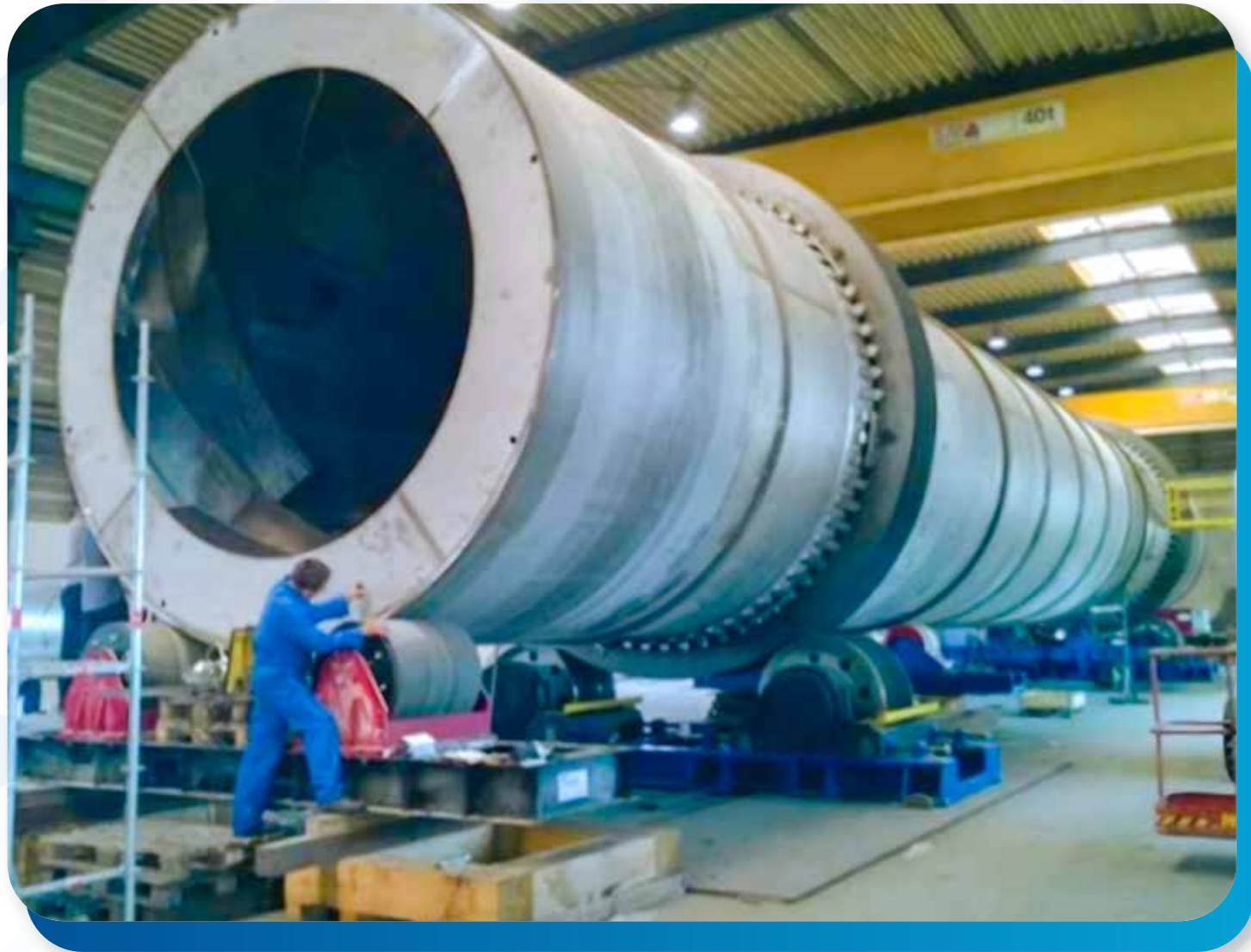
Figure 1. Big rotary drum from stainless steel at the manufacturing hall (4.5 m in diameter, 35 m length) for drying of 320 tph fertilizers.
