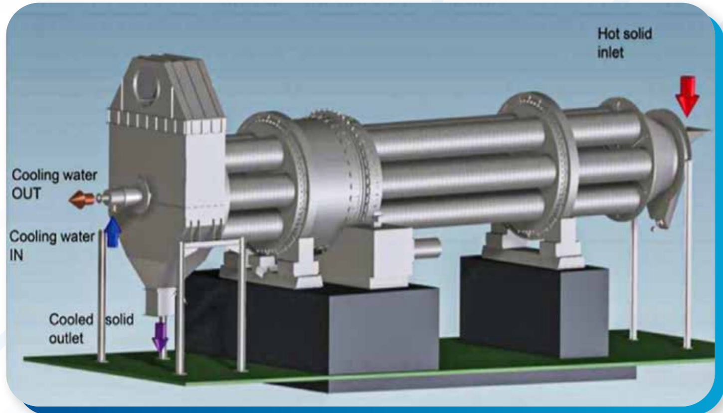
Figure 28 . Indirect planetary rotary cooler for 40 tph solid.
