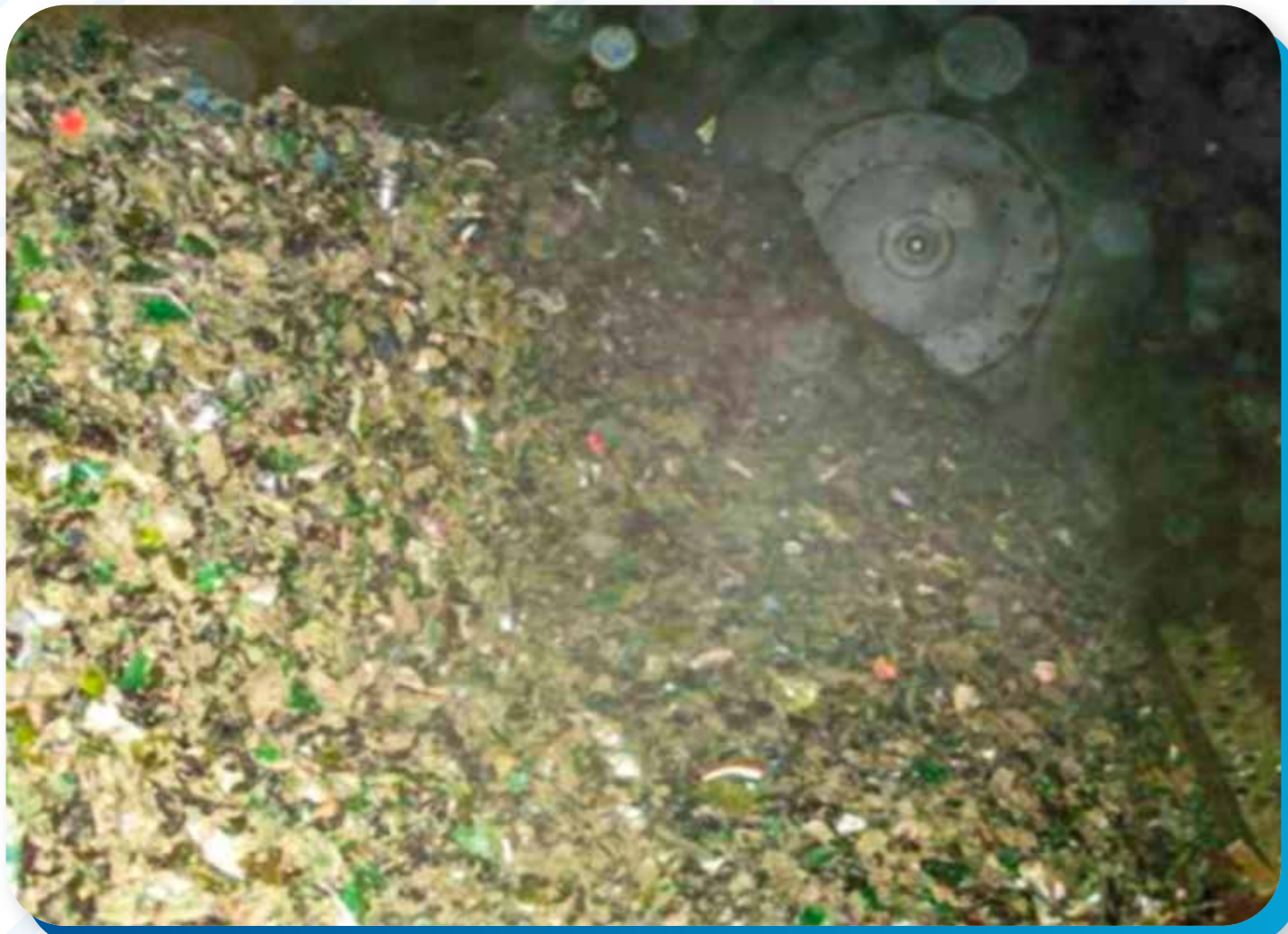
Figure 22 . View into the cleaning compartment of a combined drying cleaning drum.
