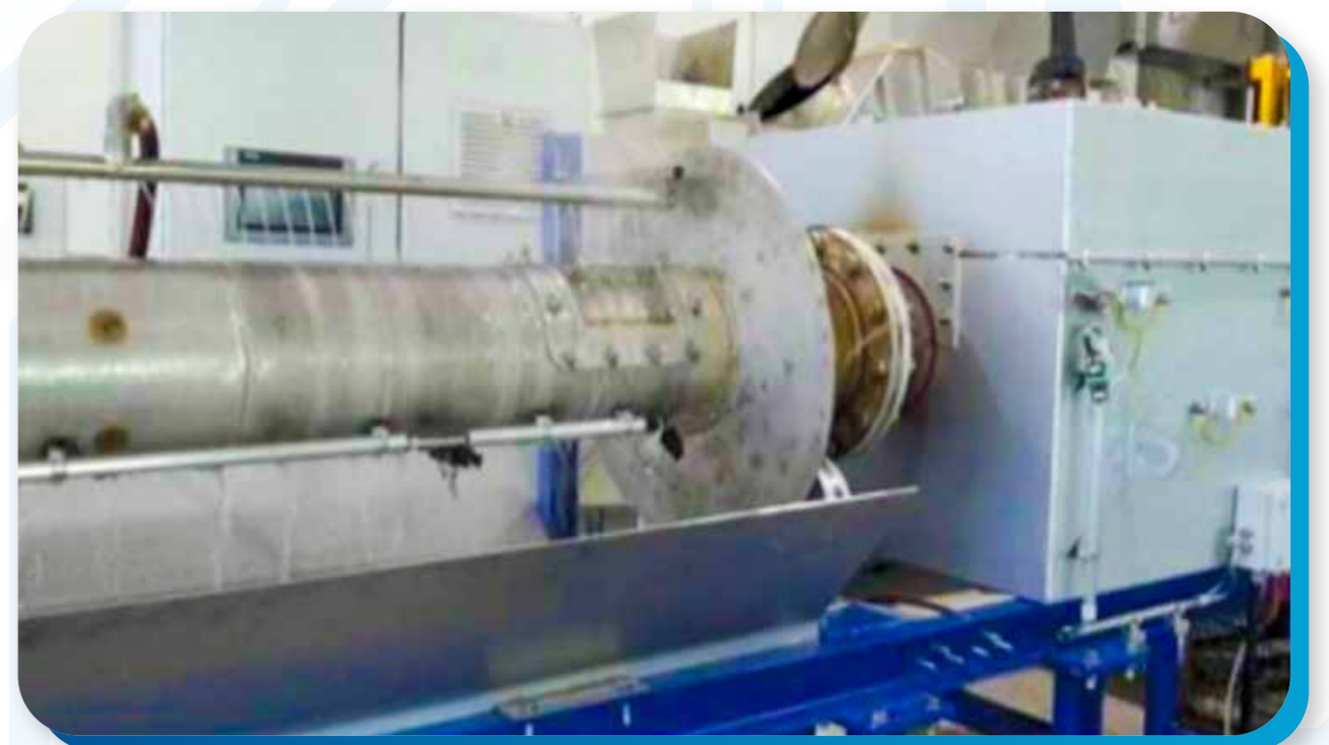
Figure 31 . Test plant for continuous solids cooling.
