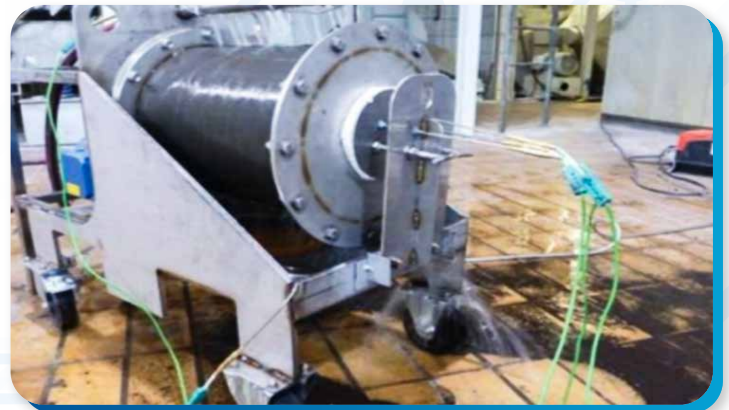
Figure 30 . Batch laboratory cooler for determining the properties of bulk materials and heat transfer of real solids.
