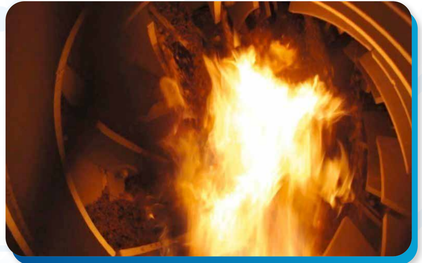
Figure 1. View into a dryer drum with flame in the interior of the drum.
