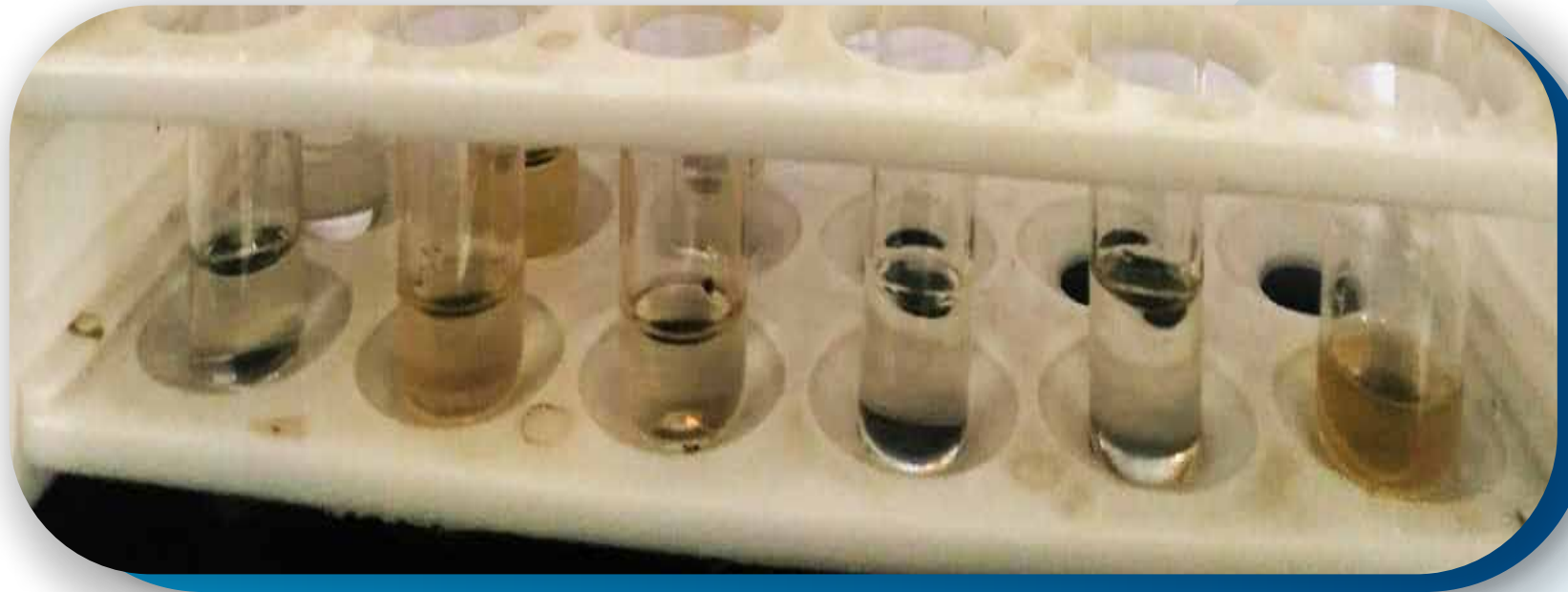
Fig. Separation of oil through chloroform phase transfer
