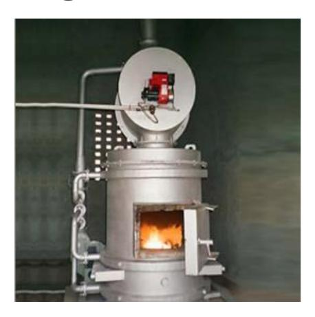
Incineration is the process of control and complete combustion, for burning solid wastes. It leads to energy recovery and destruction of toxic wastes.
