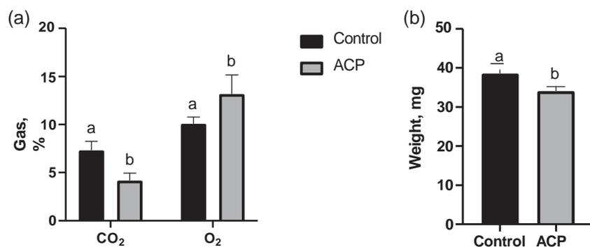
FIGURE 4 Effect of indirect 5 min of atmospheric cold plasma (ACP) treatment on (a) respiration and (b) weight of adult insects. Mean values ( $n = 6$ ) of the control group were compared with the ACP-treated group. Vertical bars indicate the standard deviation. Different letters represent significant differences at the level of  $p < .05$
