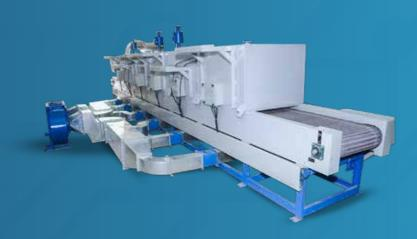
Infrared (IR) dryers are modern day industrial drying solutions for material surface, Infrared (IR) dryer uses the infrared radiations, and Infrared radiations are invisible electromagnetic radiation whose wavelength is longer than the visible light wave range between 0.78 and 1000  $\mu$ m.
