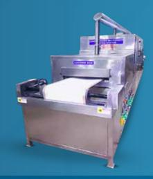
Microwave is not a type of heat, rather it's a form of energy that are exhibited as heat by the means if their interaction with the material. It results in material to heat themselves, the mechanism of energy conversion used is dipole rotation.
