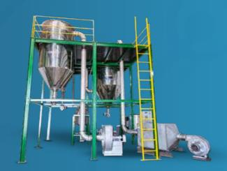
Spray drying is method of dehydrating fluids, solutions and thin slurries, it converts the fluids or slurries to powder form. Liquid or slurry material to be dehydrated is sprayed in the form of a fine droplet dispersion into hot airstream.
