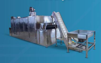
A band dryer is a continuous drying machine for materials like food, chemicals, and pharmaceuticals. It uses a conveyor belt in heated air for efficient drying, with precise temperature and airflow control to maintain product quality.
