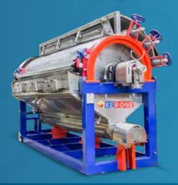
The drum dryer is very flexible in nature, its operation depends on the pressure of steam within the drum, speed of drum rotation, width of applicator and the ratio of drum speed rotations.
