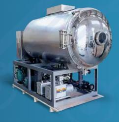
Freeze dryers, or lyophilizers, remove moisture by freezing and applying a vacuum, preserving structure and quality. Used in pharmaceuticals, food, and research, they extend shelf life and prevent thermal damage, producing light-weight, rehydratable products.
