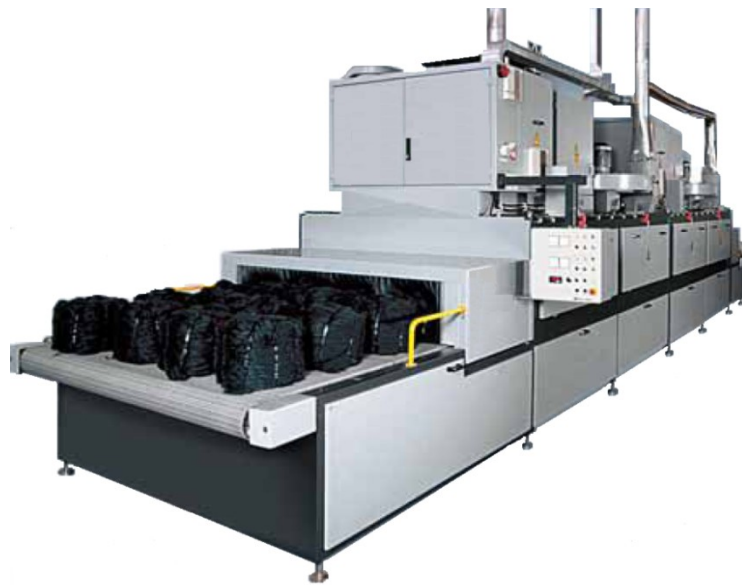
Fig.1: "RF 2x75 kW" dryer for fine wool tops in 10 Kg bump form, dyed and hydro-extracted on stainless steel spindles and loaded manually to the dryer.
