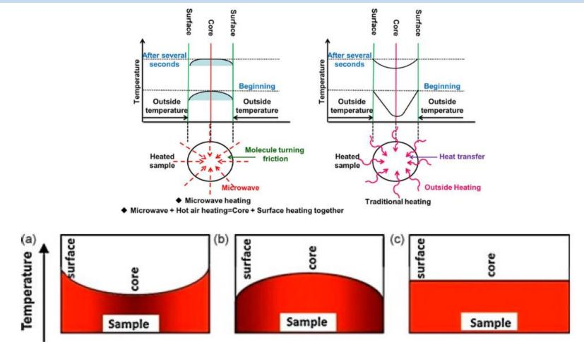
Temperature profile within the sample in: (a) conventional heating; (b) microwave heating; and (c) microwave hybrid heating
