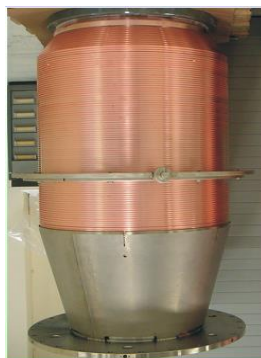
2.2 MW, CW collector
