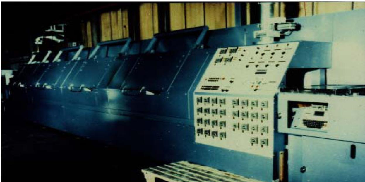
***Fig. 9 Modular microwave pre-heater for rubber vulcanisation***
